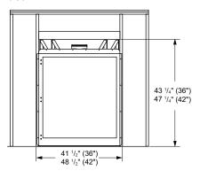
Figure 4 - Framing Clearances with Outside Air Flex Duct
